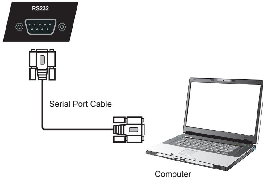
After using serial port cable to connect central control equipment and machine, certain function of the machine can be controlled via central control equipment, such as: machine ON/OFF, and adjustment of sound volume, etc.
