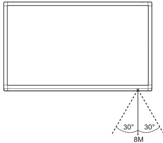
Remote control can work normally within the range of 8 meters distance, 30 degrees left and right from the remote control receiver; in order to protect environment, please dispose waste battery into recycling box.
